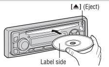
Playback will start automatically after recognizing the data of the loading disc.
