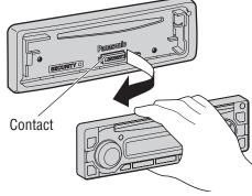
Gently press the bottom of the case and open the cover. Place the face plate into the case and take it with you when you leave the car.
